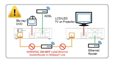
An Ethernet switch, wired or wireless router, or modem can be safely connected to the black colored Ethernet ports on the PLX-HDB.4, labelled "10Base-T/100Base-T ETHERNET". This enables distribution of Internet/Ethernet data throughout the HD-AV system, with the PLX-HDB.4 in effect acting as a 6-port Ethernet switch; 3 ports at the TX and 3 ports at the RX, with up to 100m CAT6 cable in between.
